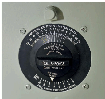
Located in the extreme right quadrant of the overhead panel, the mechanical fuel flow calculator never used in airUK ops
