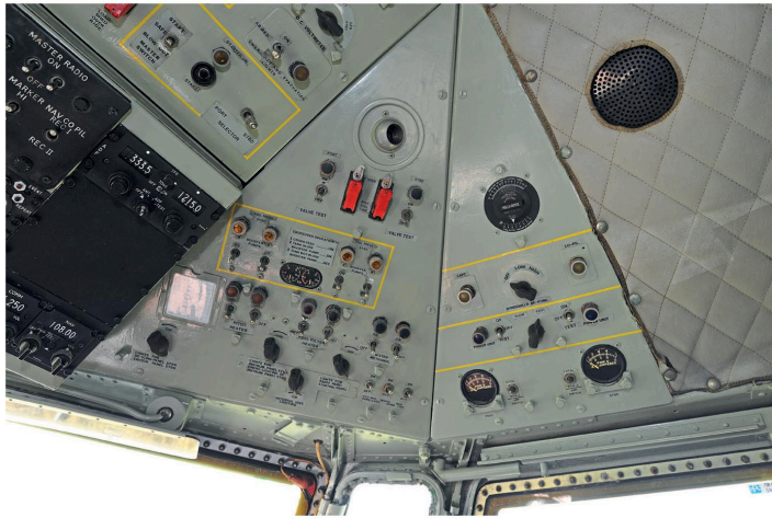
Overhead panels in what was otherwise a very WWI-era cockpit include the engine start switches
