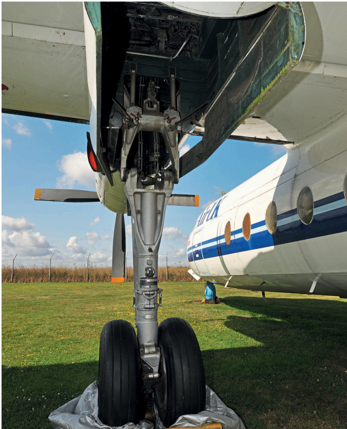
▲ Seen here on surviving airUK F.27-200 Friendship G-BHMY, the port main undercarriage leg and doors ▶ Preserved at the City of Norwich aviation museum and 'looking for all the world as if it's ready to go out on its next service', MY's cockpit
