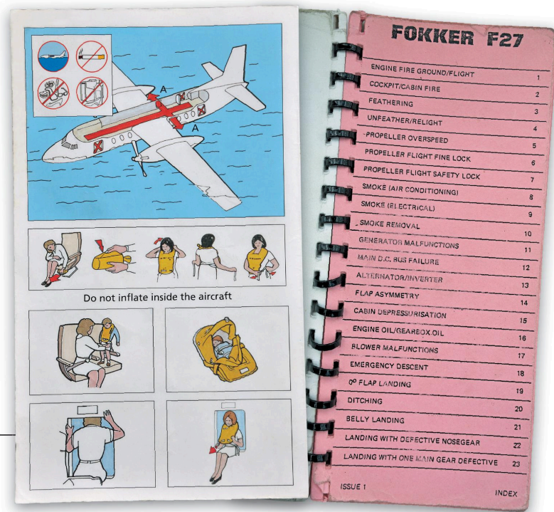
Passengers were instructed to escape via the underwing hatches only after ditching and the emergency checklist was brief by today's standards
